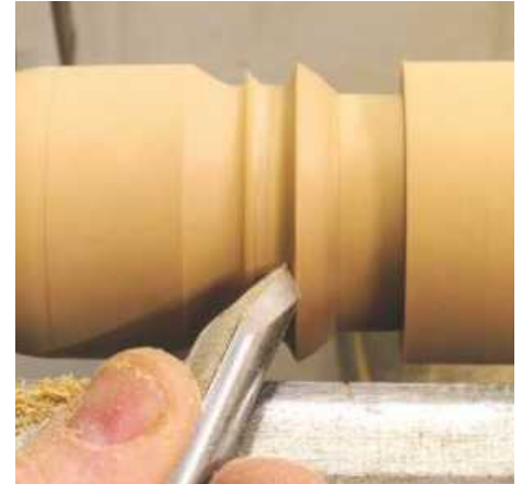
▲ Pic.21 The next two photos show the importance of getting the tool in the correct position to make the cut. The bevel or cutting angle of the gouge is at right angles to the work; this will give an almost undercut look to the top
